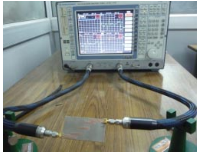
Figure 3 : Setup for measurement of S parameters of proposed filter.
