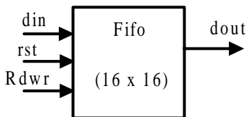
Figure 2 : Realization of 16 x 16 fifo logic for coefficient interface
